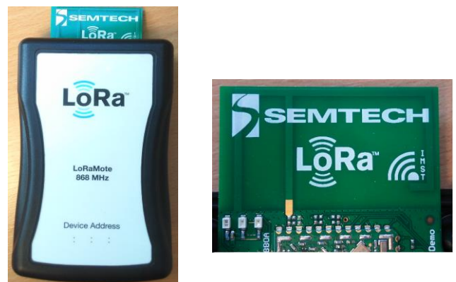
Fig. 1. Semtech LoRamote device used for testing including the inverted-F antenna
