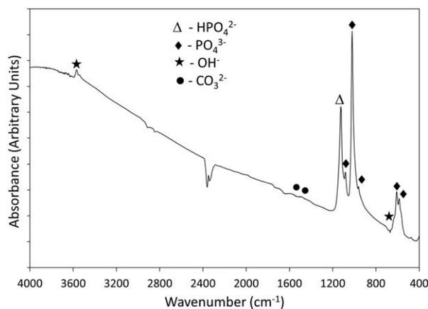
**FIGURE 1.** FTIR Spectrum for CaP-TiTi sample.
