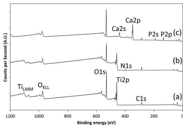
**FIGURE 3.** XPS wide energy survey scans (WESS) for (a) abraded chemically pure titanium surface (cpTi), (b) titanium layer sputtered onto a cpTi surface (TiTi), and (c) CaP coating on TiTi surface (CaP-TiTi).
