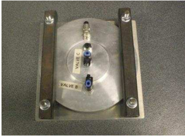
3 4 (c) Clamped test heads to confirm water tightness
