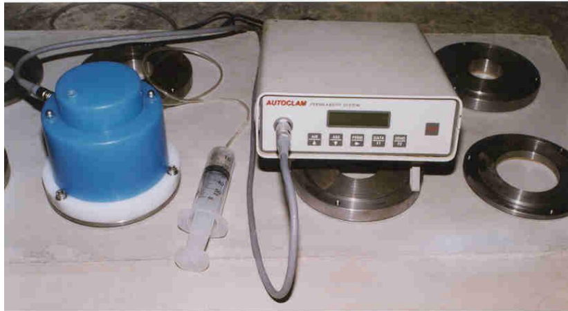
(a) Autoclam permeability system, including 50 and 75mm internal diameter test rings and syringe for applying air pressure
