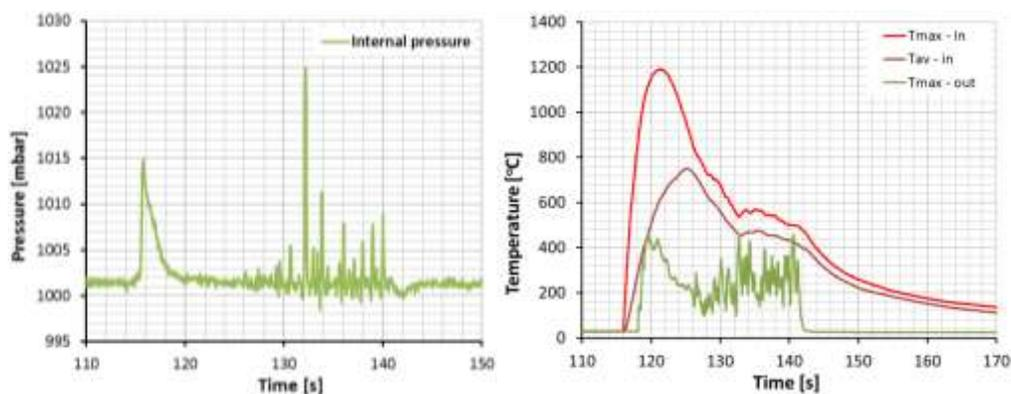
**Figure 9.** Typical pressure transients (left) and temperature histories (right) for under-ventilated jet fire regime (Test 61: release of hydrogen 1.086 g/s, lower vent area of size 3x30 cm<sup>2</sup>).
