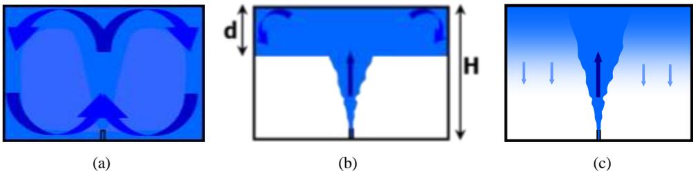
**Figure 1.** Regimes of light gas dispersion: (a) fully homogeneous ( $Ri_v < 0.0025$ ); (b) stratified with a homogeneous layer ( $0.0025 < Ri_v < 3$ ); (c) stratified well-mixed layer ( $Ri_v > 3$ ) [12-14].
