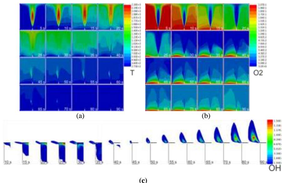
**Figure 4.** Under-ventilated jet fire in Test No.7: (a) temperature profile; (b) O<sub>2</sub> concentration profile; (c) external OH concentration profile.
