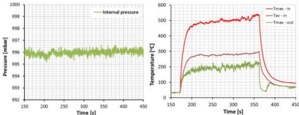
**Figure 7.** Typical pressure transients (left) and temperature histories (right) for well-ventilated jet fire regime (Test 25: release of hydrogen 0.1086 g/s, upper vent area of size 30x3 cm<sup>2</sup>).
