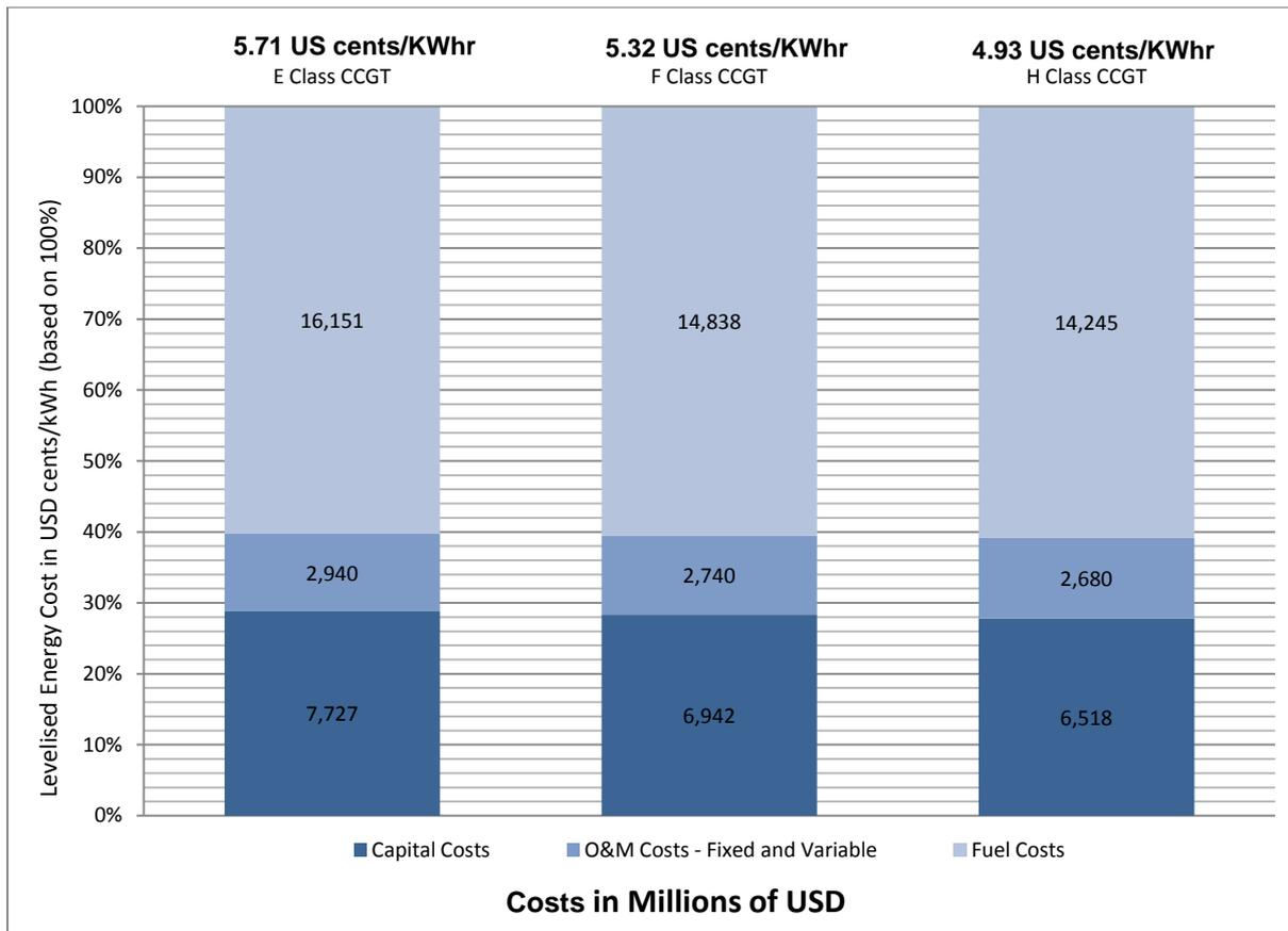
Figure 3 LCOE for each CCGT Technology in \$ cents/kWh (based on 100%)
