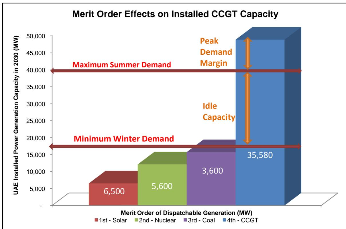
Figure 9 Merit order effects on installed CCGT capacity
