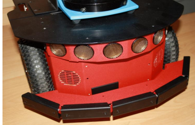
Figure 3. Pioneer P3DX fitted with the Polaroid Sonar Array (front and rear). There is also a Bumper Array fitted.
