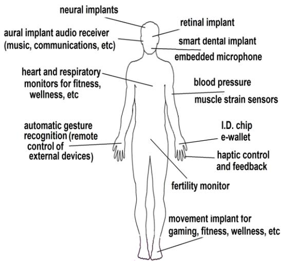
Fig. 1. Target areas for implantable body-area network technologies.
