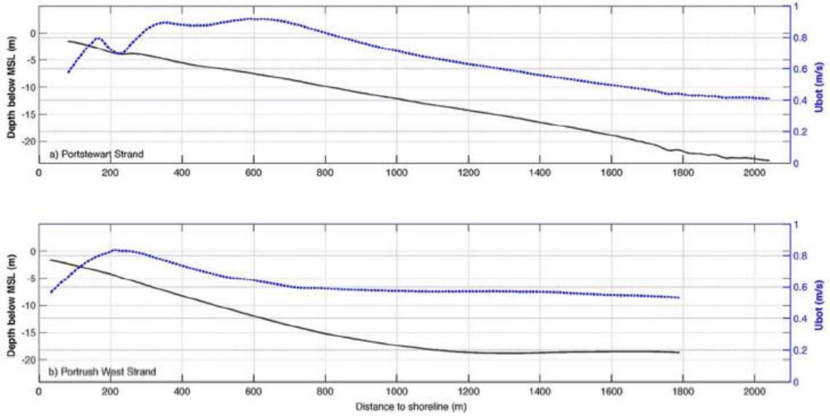
**Figure 8.** Near bottom maximum orbital velocities (dashed blue line) along the nearshore profile (solid grey line) of Portstewart Strand (a) and Portrush West Strand (b). Modelled  $U_{bot}$  values for the peak storm conditions at 00:00 of June 22<sup>nd</sup>.
