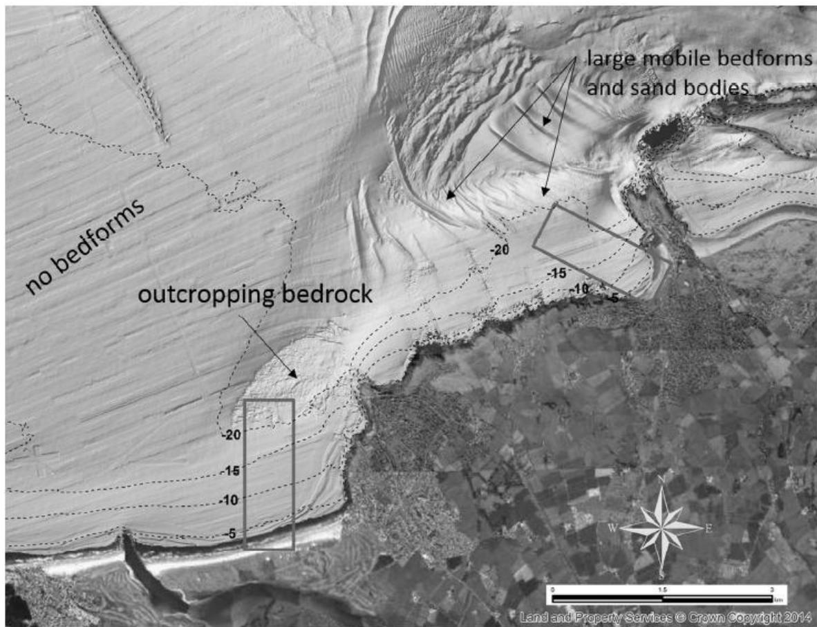
**Figure 9.** JIBS high-resolution multibeam bathymetry data collected in 2007. Note the presence of large sand bodies and mobile bedforms offshore of West Strand, seaward of 20 m depths, compared to the lack of bedforms and presence of outcropping bedrock at Portstewart.
