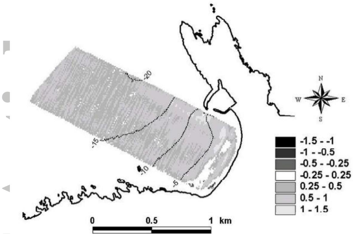
**Figure 5.** Storm-associated bathymetric difference map for West Strand, generated by comparing June 11th and June 26th, 2006 survey data. Note extensive shoreface-wide deposition attributed to the high-energy event, with minimal areas of erosion.
