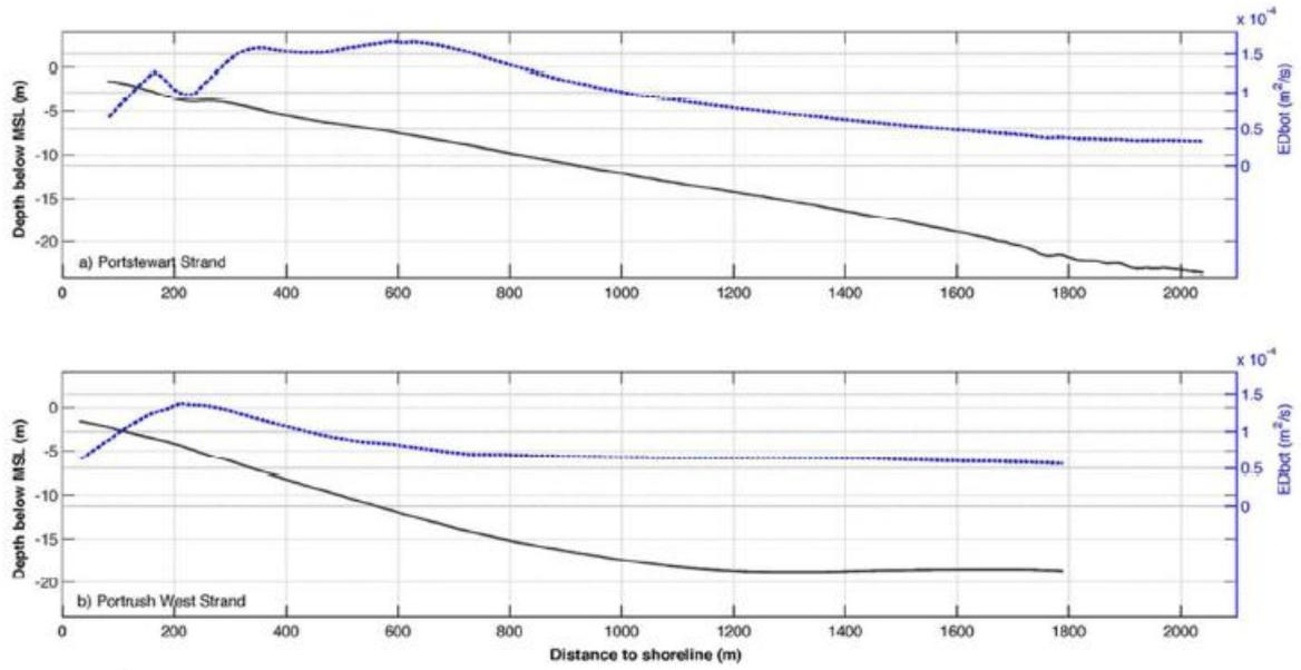
**Figure 7.** Energy dissipation due to bottom-friction (dashed blue line) along the nearshore profile (solid grey line) of Portstewart Strand (a) and Portrush West Strand (b). Modelled  $ED_{\text{bot}}$  values for the peak storm conditions at 00:00 of June 22<sup>nd</sup>.
