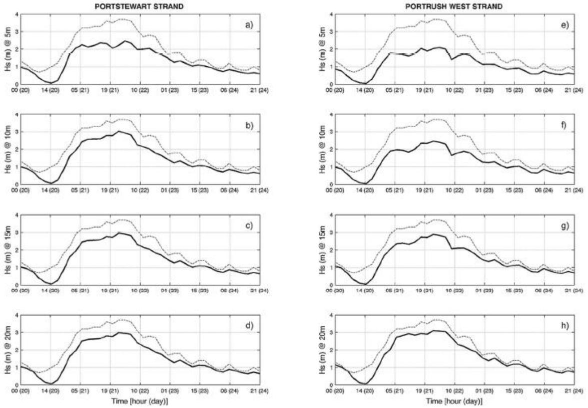
**Figure 6.** Time-series of nearshore wave height in the shoreface of Portstewart Strand (left panels) and Portrush West Strand (right panels), at 5 m, 10 m, 15 m and 20 m depths (offshore conditions displayed as dashed line).
