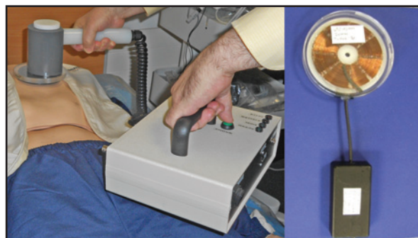
TOP: In the lab at the University of Ulster, a team member illustrates use of the hand-held external transmitter PIAD module that provides power to the implanted defibrillator. BOTTOM: Left: The external module also wirelessly receives sensor data from the implanted defibrillator. Right: The implantable unit, capable of delivering cardioversion shocks and sensing various parameters of the myocardium (e.g. ECG, electrical impedance spectrum, temperature)
