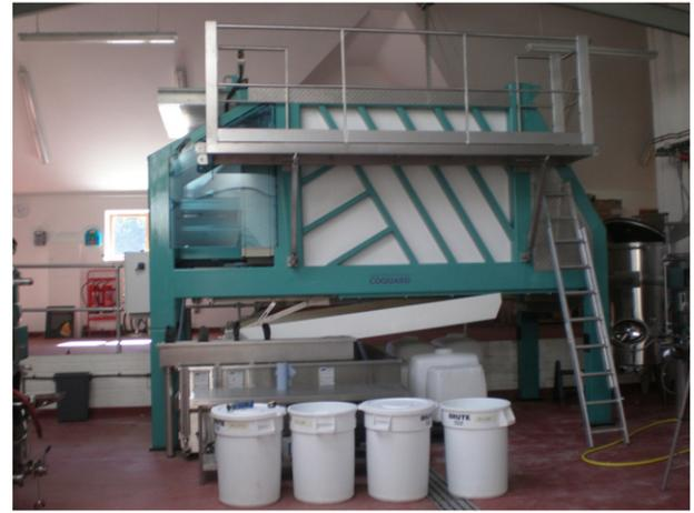
Fig. 8. Grape processing equipment representing a high power rating but relatively low energy usage.
