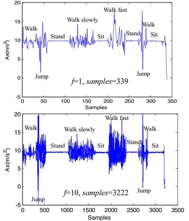
Figure 2. Comparison of acceleration  $Ax$  signals and activity classification results between  $f = 1$  and  $f = 10$ . The sample number was 339 vs 3222 for 5 minutes data recording, however the posture classification results shown in both figures were same that classified and marked using SVM model automatically in Matlab environment.
