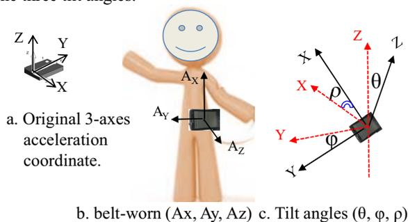
Figure 3. Three tilt angles for measuring tilt postures.
