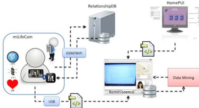
**Figure 1.** Architecture of the R<sup>3</sup>S System detailing the information flow from the wearable life-logger (*miLifeCam*) to the database (relationshipDB) containing all social contact information..
