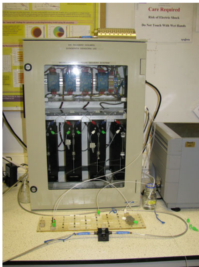
Figure 4 – Photograph of the assembled prototype fluid delivery system, with the microfluidic breadboard system shown in the lower portion of the photograph.
