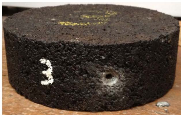
Figure 1. Test specimen with hole drilled to determine temperature internal temperature
