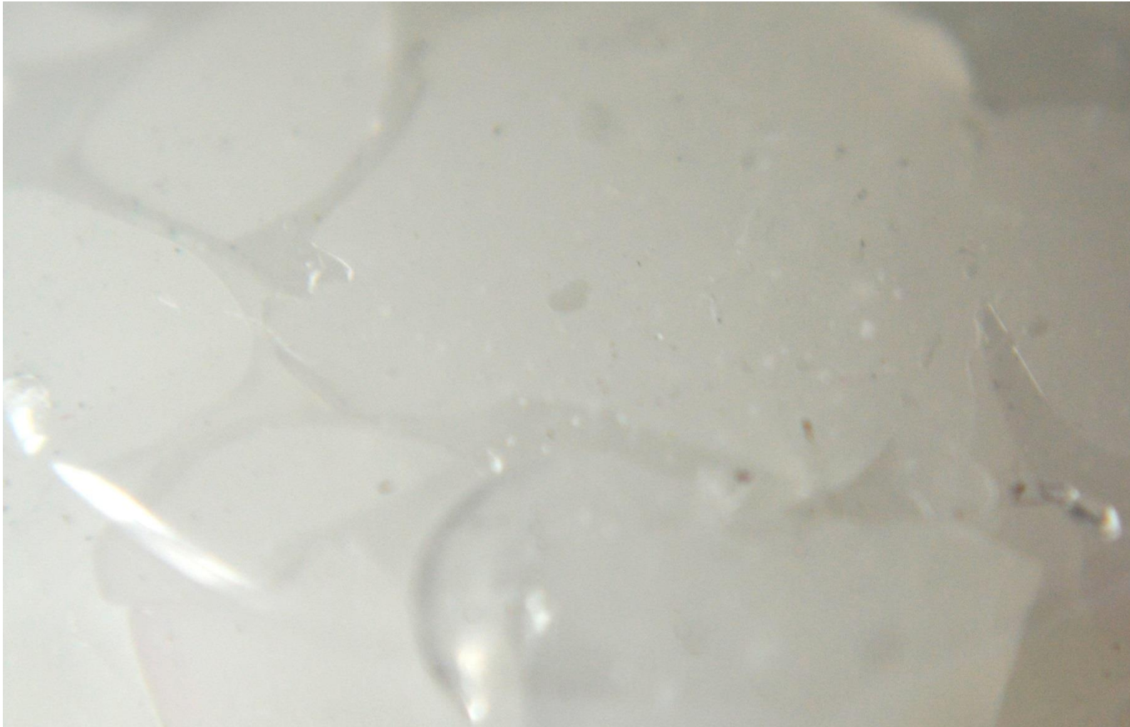
Fig. 13 Cluster marker close up showing air spaces
