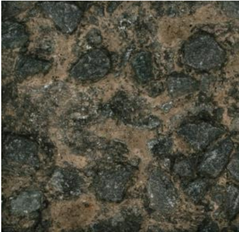
Figure 10. Original digital image of the 14mm chip seal
