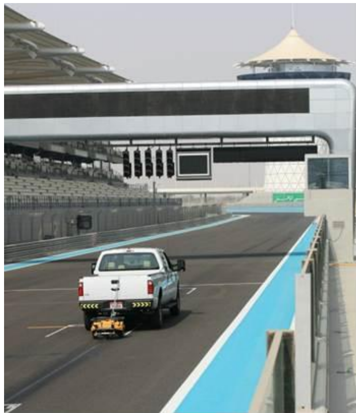
Figure 7 – GripTesting at Yas Marina, Abu Dhabi
