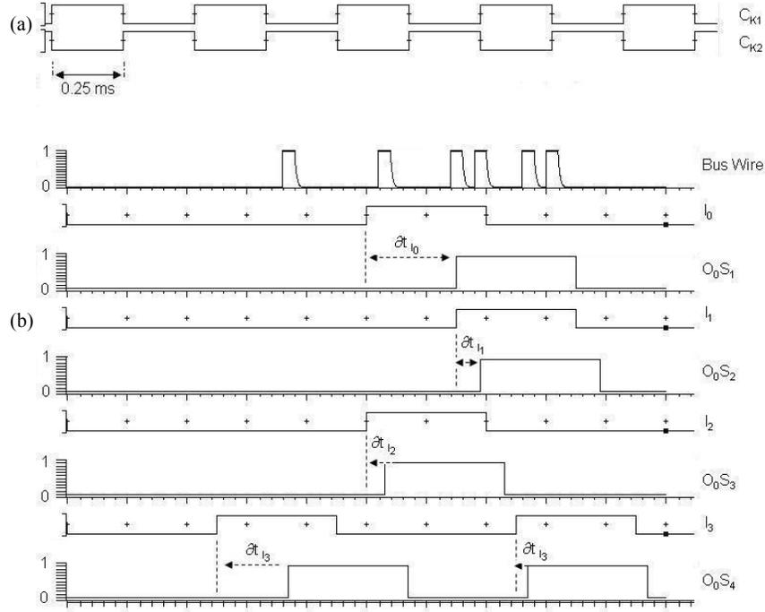
**Fig. 3.** (a) Timing diagram where the clock signal to the output sampling D-latches,  $D5-D12$ , is delayed by 0.25ms, quarter of the sampling pulse period. (b) bus wire signals caused by random firing neurons  $I_0 - I_3$ , and  $O_0S_1 - O_0S_4$ , show the time of arrival of pulses at the appropriate synapses
