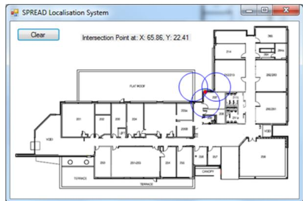
Figure 2: Prototype illustrating 'lost' device being localized.
