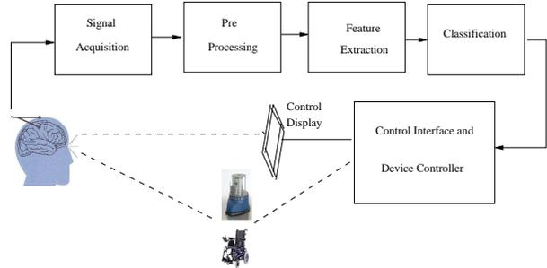
Fig. 1. Basic Design of a simple BCI system
