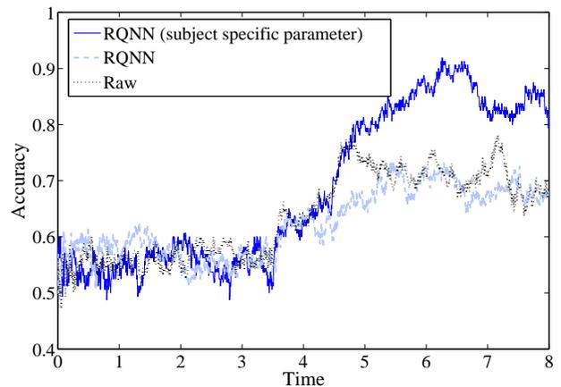
Fig. 15. CA plot for the subject 0503T on the raw EEG and the RQNN filtered EEG (on subject independent and PSO tuned subject specific parameter) using the LDA classifier
