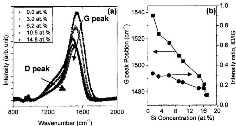
FIG. 2. (a) Normalized and background subtracted visible-Raman spectra and (b) fitting parameters [intensity ratio ( $I_D/I_G$ ) and G peak position] of Si-*a*-C:H films as a function of Si content.
