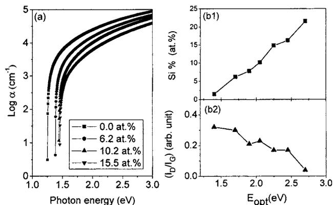
FIG. 5. (a) Optical-absorption edge vs photon energy as a function of Si content. (b1) The effect of Si incorporation on the optical band gap ( $E_{opt}$ ) and (b2) Raman  $I_D/I_G$  ratio of a series of Si-*a*-C:H films.
