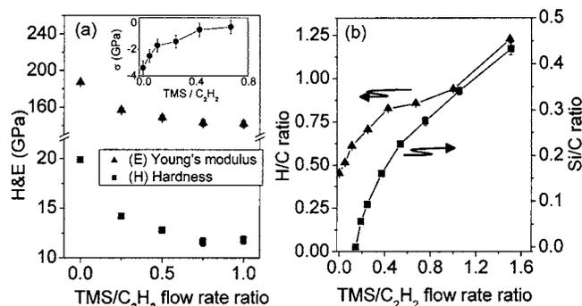
FIG. 6. The effect of Si incorporation on (a) Young's modulus ( $E$ ) and hardness ( $H$ ) of *a*-C:H films. The inset illustrates the reduction of residual stress of the PECVD films as a result of the TMS-incorporation process. (b) The evolution of H/C and Si/C concentrations vs TMS/C<sub>2</sub>H<sub>2</sub> flow-rate ratio.
