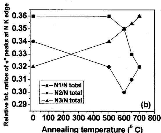
FIG. 6. (a) Variation of N  $K$  edge spectra of a ta-CN film containing 12.5 at. % N with annealing temperature. (b) Variation of relative intensity ratios of  $\pi^*$  peak at N  $K$  edge with annealing temperature.
