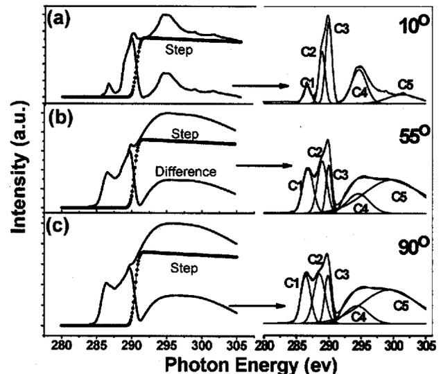
FIG. 4. Deconvoluted C K peaks for angles (a)  $10^\circ$ , (b)  $55^\circ$ , and (c)  $90^\circ$  deg, respectively, of a ta-CN film containing 12.5 at. % N. On the left compartment the solid line represents the resulting difference curve and the dotted line the fitted ionization step function.
