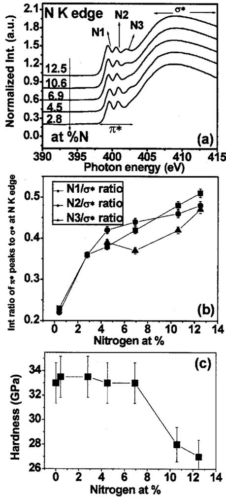
FIG. 2. (a) Variation of N K edge spectrum with nitrogen concentration in the films. (b) Intensity ratio of  $\pi^*/\sigma^*$  peak at N K edge with nitrogen concentration. (c) Variation of film hardness with nitrogen concentration.
