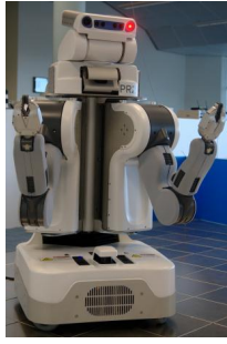
Fig. 2. The mobile manipulator platform PR2. The robot has two 7DOF arms and an holonomic base. The pan-tilt head unit is equipped with two stereo cameras, one high resolution camera and one texture projector (the red light). A tilting laser and a fixed laser on the base are used for navigation and motion planning.
