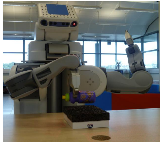
Figure 13: The PR2 while stacking a bottle over a box. The robot was controlled by the FSA in Figure 11.
