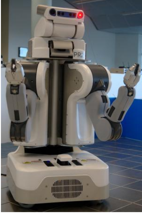
Figure 5: The mobile manipulator platform PR2. The robot has two 7DOF arms and an holonomic base. The pan-tilt head unit is equipped with two stereo cameras, one high resolution camera and one texture projector (the red light). A tilting laser and a fixed laser on the base are used for navigation and motion planning.
