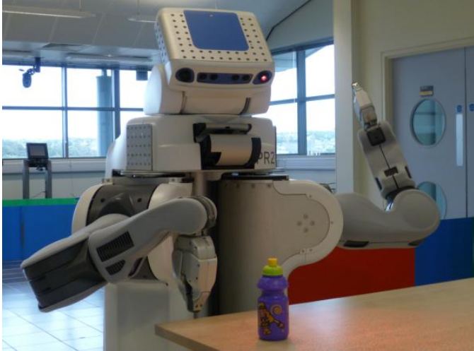
Figure 8: The PR2 while pushing an object. Several random object's positions were tested, and the robot had to use both arms.
