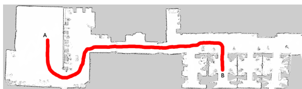
Fig. 3. The map of the environment where the experiments were conducted. The users had to drive the robot from point A to point B and back. The entire path length is around 60m. The robot footprint is represented by the width of the red path shape.
