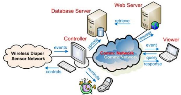
Figure 2. Overview of iCMS Functional Software Components
