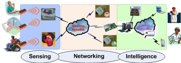
Figure 1. Overview of 3-Tier System Architecture of iCMS
