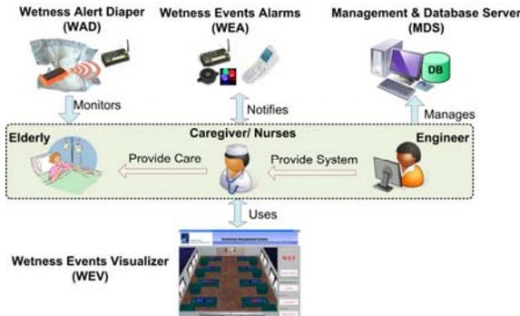
Figure 4. Overview of iCMSv1 Components and Interactions
