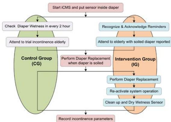
Figure 12. Trial Protocol and Operations with iCMSv2
