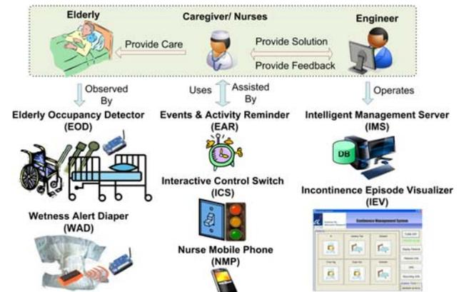
Figure 13. Overview of iCMSv2 Components and Interactions
