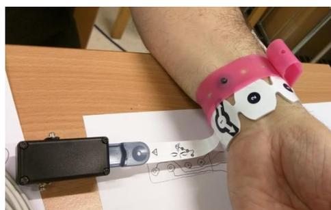
Figure 3. BIS-Quatro sensor strap with fixing dry electrodes elastic band on the wrist.
