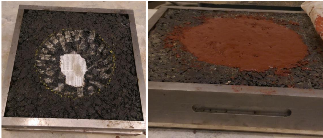
Figure 6. Simulated pot hole before and after repair with geopolymer cement concrete
