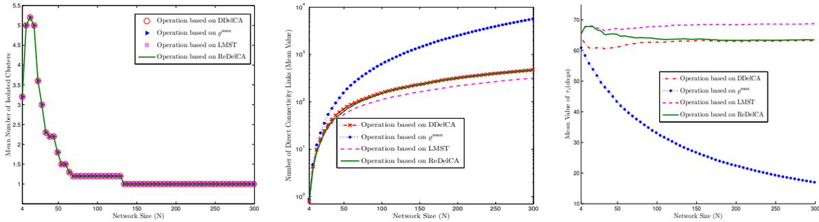
Fig. 4. Simulation results: The mean value of isolated clusters (left), the mean value of direct connectivity links (middle), the mean lifetime per node (right) for  $f_{RX} = f_{TX} = 1000$ bps, versus the network size  $N$ .
