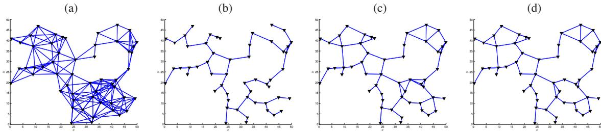
Fig. 3. The connectivity status of a network comprised of  $N=54$  nodes, resulting from the transmission power configuration based on (a) static / maximum transmission power, (b) the LMST, (c) the DDeICA and (d) ReDeICA.
