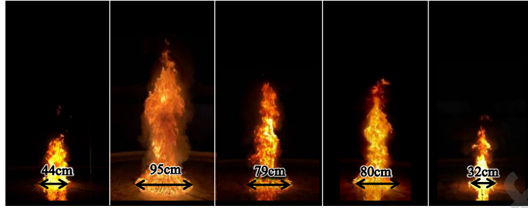
Fig. 3. Images of continuous spill fire at different times after discharge in Test 8.
